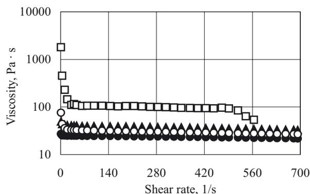
Fig. 2. Melt viscosity (at 120 °C) versus shear rate of UP modified with various clay additives;  $\bullet$  — unmodified,  $\square$  — C30B,  $\blacktriangle$  — C15A,  $\circ$  — MMT-Na
