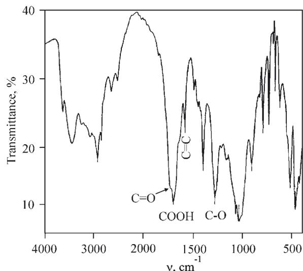
Fig. 3. FT-IR spectrum of clay MMT-ADA modified by the reaction with epichlorohydrine, maleic anhydride and phthalic anhydride
