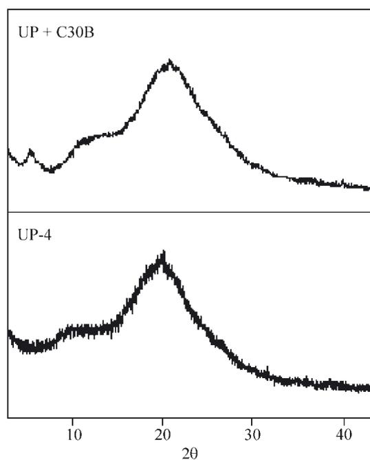
Fig. 4. XRD diffractograms of physical blend of unsaturated polyester with organoclay (UP + C30B) and unsaturated polyester synthesized in the presence of organoclay (UP-4) composition
