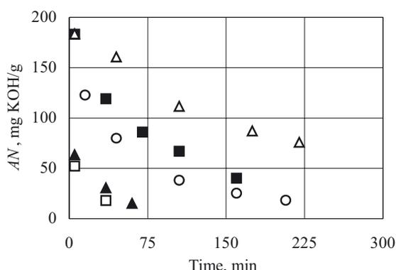
Fig. 1. Time dependence of acid number (AN) of UP synthesized in the presence of various clays; ■ — unmodified resin,  $\Delta$  — MMT-ADA,  $\circ$  — MMT-Na,  $\blacktriangle$  — C15A,  $\square$  — C30B
