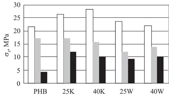
Fig. 4. Comparison of tensile strength of biocomposites with wood flour or kenaf, determined at various temperatures: □ – 23 °C, ■ – 40 °C, ■ – 60 °C
