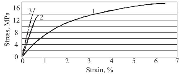
Fig. 3. Comparison of tensile curves (stress-strain) for PHB filled with wood flour or kenaf fiber determined in 40 °C: 1 – PHB, 2 – PHB filled with wood flour, 3 – PHB filled with kenaf fiber
