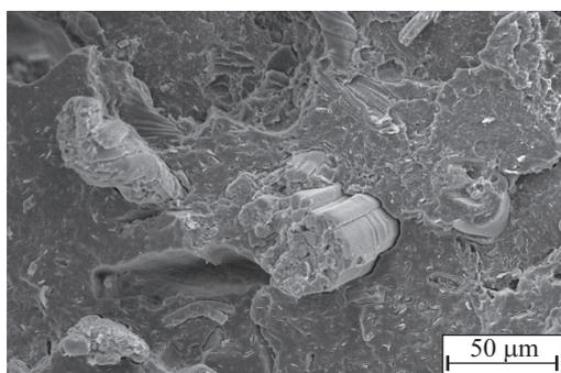
Fig. 7. SEM image of fracture at ambient temperature after elongation of PHB filled with 40 wt. % of kenaf fiber
