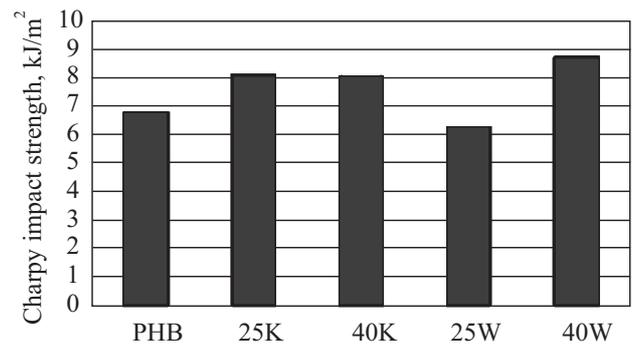
Fig. 1. Comparison of Charpy impact strength for PHB and biocomposites with wood flour or kenaf
