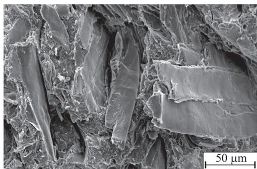
Fig. 8. SEM image of fracture at ambient temperature after elongation of PHB filled with 40 wt. % of wood flour
