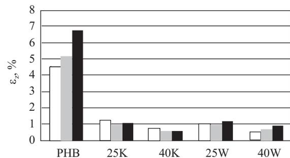
Fig. 6. Comparison of strain at break of biocomposites with wood flour or kenaf, determined at various temperatures: □ – 23 °C, ■ – 40 °C, ■ – 60 °C
