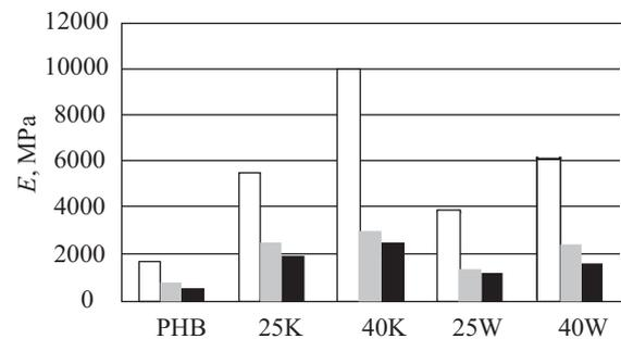
Fig. 5. Comparison of modulus of elasticity of biocomposites with wood flour or kenaf, determined at various temperatures: □ – 23 °C, ■ – 40 °C, ■ – 60 °C
