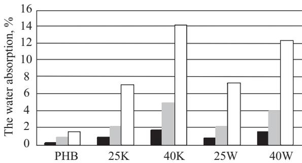
Fig. 2. Comparison of water absorption by PHB and biocomposites with wood flour or kenaf: ■ – samples soaked for 24 hours, ■ – samples soaked for 7 days, □ – samples soaked for 90 days
