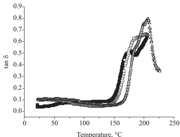
Fig. 7. Heating (■ – 21 → 205 °C) – cooling (○ – 205 → 21 °C) – heating (Δ – 21 → 226 °C) cycle for the polyesteramide (IIIe)
