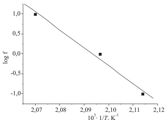
Fig. 9. Arrhenius plot corresponding to glass transition of polymer (IIIe) ( $y = 93.89 - 44845.68x$ )
