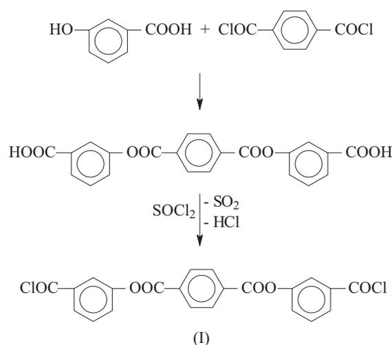
Scheme A. Synthesis of the diester-diacid chloride (I)
