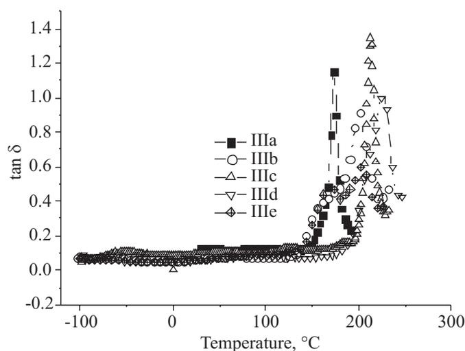
Fig. 6. Loss tangent ( $\tan \delta$ ) vs temperature of the polyesteramides at 1 Hz
