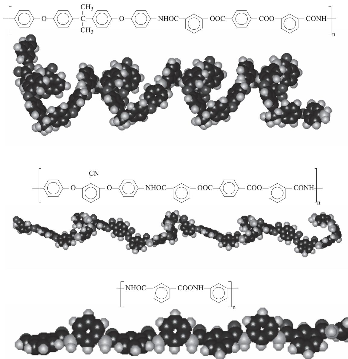
Fig. 2. Model molecules (four repeating units) for polyesteramides (IIIc) and (IIIb) and aromatic polyamide
