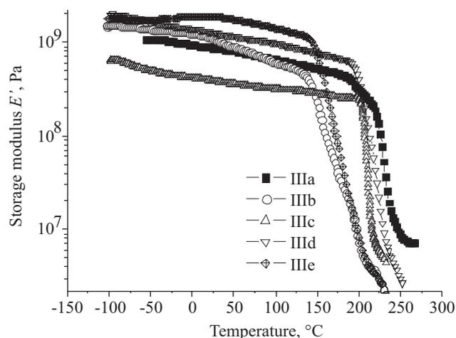
Fig. 5. Dynamic storage modulus vs temperature of the polyesteramides (III) at  $1$  Hz
