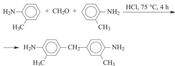
Scheme B. Synthesis of 4,4'-diamino-3,3'-dimethyldiphenylmethane (IIb)
