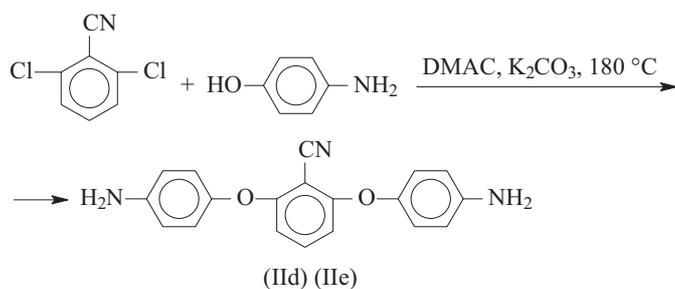
Scheme C. Synthesis of 2,6-bis(*p*-aminophenoxy)-benzotrile (II<sub>d</sub>), (II<sub>e</sub>)
