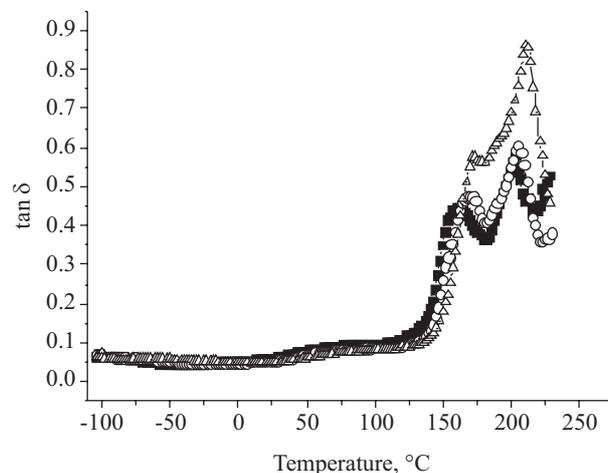
Fig. 8. Loss tangent ( $\tan \delta$ ) vs temperature of polyesteramide (IIIe) at three frequencies: 0.1 Hz (■), 1 Hz (○) and 10 Hz (Δ)
