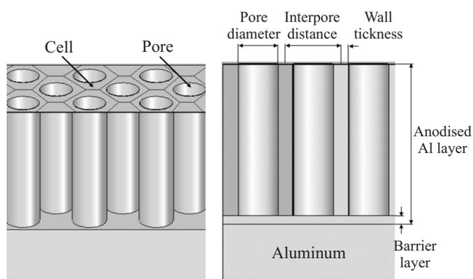
Fig. 5. Anodized aluminum structure
