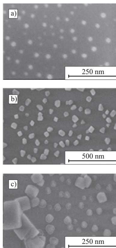
Fig. 2. SEM images of YAB nanoparticles obtained as a first fraction – 50 nm (a) after separation, second fraction – 100 nm (b) and before separation process (c)
