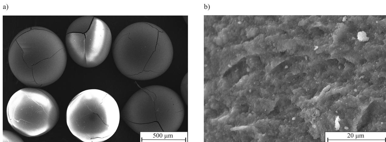
Fig. 1. SEM images of hybrid polymer containing iron oxide
