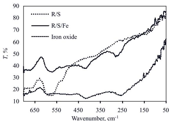
Fig. 2. Far infrared spectra of polymer matrix – sulfonamide S/DVB copolymer – R/S, hybrid polymer containing iron oxide – R/S/Fe and iron oxide obtained by oxidation of Fe(II) with NaOCl
