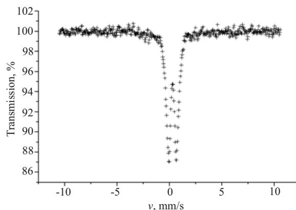
Fig. 3. Mössbauer spectrum of hybrid polymer R/S/Fe recorded at 25 °C
