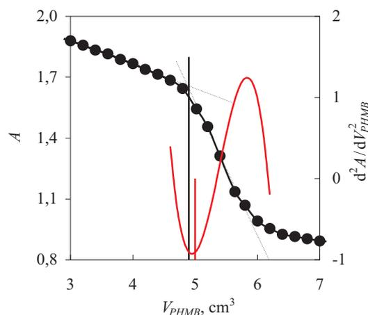
Fig. 8. The illustration of graphic methods of the endpoint determination for reverse titration (black lines — tangent method, red lines — second derivative method)
