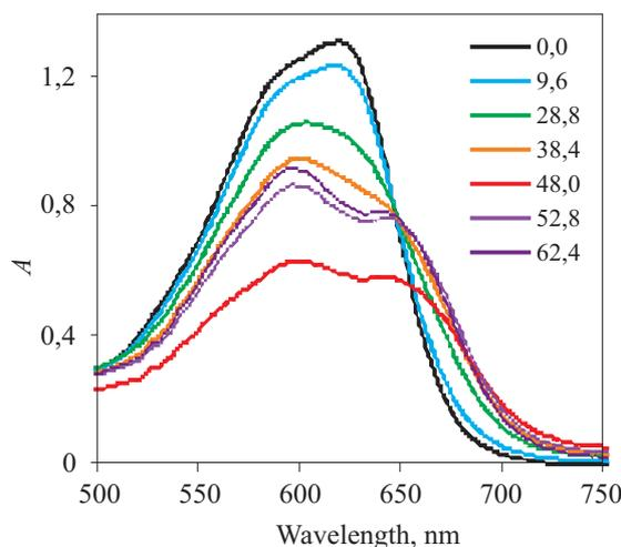
Fig. 1. UV-Vis spectra of NBB-PHMB mixtures obtained for 25 μmol/dm<sup>3</sup> solution of NBB and the indicated PHMB concentrations (given in μmol/dm<sup>3</sup> of mers)
