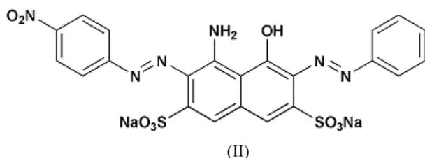
The present paper describes application of Naphthol Blue Black (NBB) dye [formula (II)] for colloid titration of PHMB in aqueous solutions. The NBB diazodye (known also as Amido Black 10B) is known as an analytical reagent for determination of proteins in biochemistry [17, 18] and detection of blood traces in forensics [19]. The proposed method is based on complexation of the anionic dye with the cationic polymer resulting in spectral changes.
