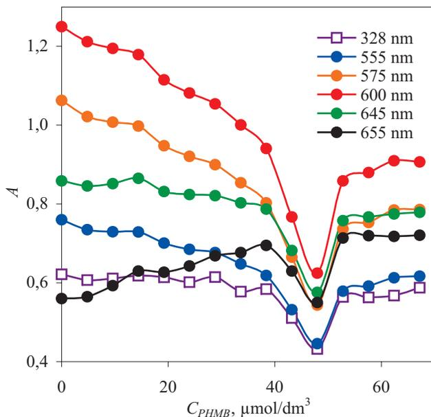
Fig. 3. Dependences of absorbance ( $A$ ) determined at various wavelengths on PHMB mers concentration ( $C_{PHMB}$ ) in solutions containing  $25 \mu\text{mol}/\text{dm}^3$  of NBB dye
