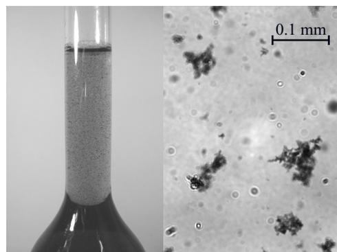
Fig. 2. Photography of NBB-PHMB suspension, which is formed at dye-to-polymer mers molar ratio equal to 1:2 (left) and micro-photograph of sediment (right)
