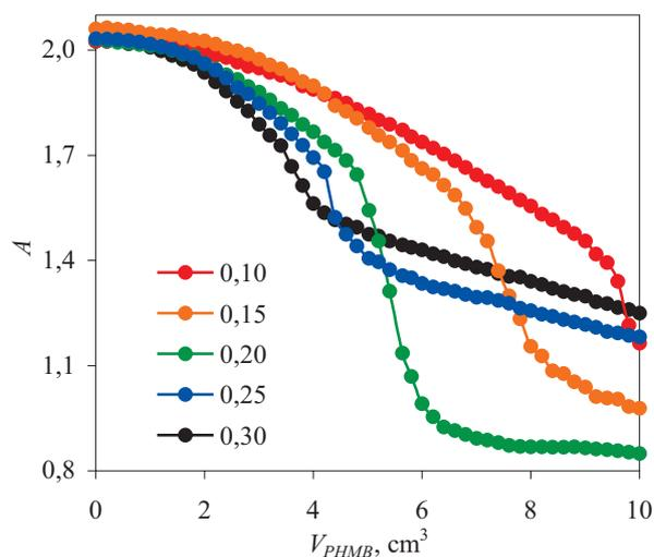
Fig. 7. Spectrophotometric reverse titration curves obtained for different PHMB mers concentrations (given in  $\text{mmol/dm}^3$ ) in the analyzed solution using the dye solution with constant concentration
