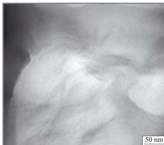
**Fig. 3.** TEM image of the mixture of silicone rubber Lukopren N1000 + Cloisite 15A (5 phr)
