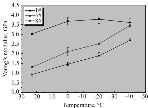
Fig. 6. Young's modulus of specimens: 1#, 6#, 8# at different temperatures
