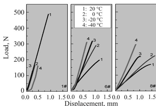
Fig. 2. Load versus load point displacement of specimens: a) 1#, b) 6#, c) 8#
