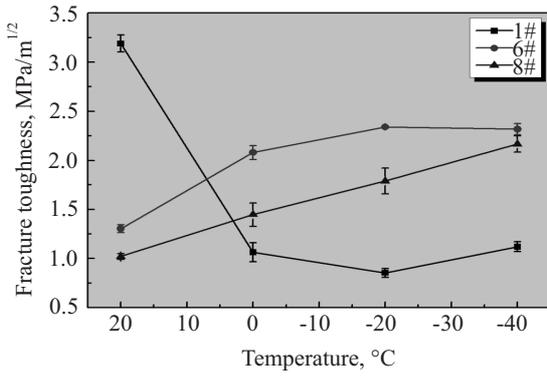
Fig. 3. Fracture toughness of specimens: 1#, 6#, 8# versus temperature
