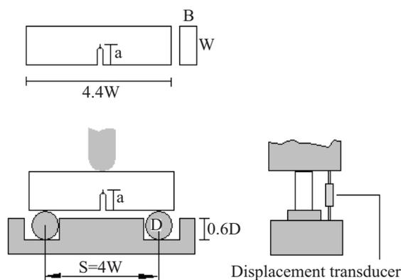
Fig. 1. Bending rig with transducer for SENB
