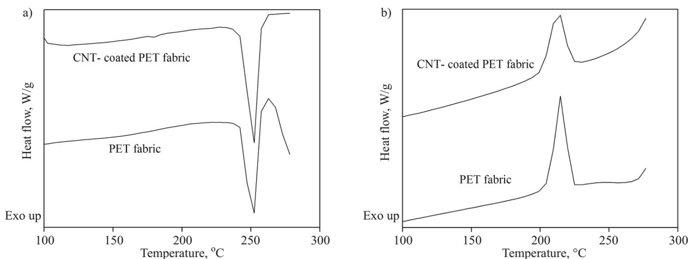
Fig. 5. DSC thermograms for PET fabric (sample 5) and  $\text{NH}_2$ -MWCNT coated PET fabric (sample 3): a) heating cycle, b) cooling cycle
