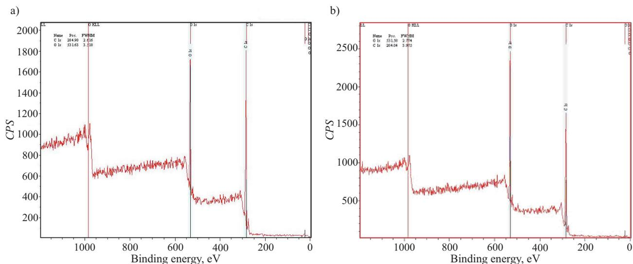
Fig. 4. Overall XPS scan survey of: a) the pristine PET fabric (sample 5), b)  $\text{NH}_2$ -MWCNT coated fabric (sample 3)
