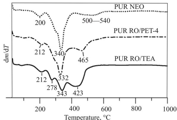
**Fig. 4. DTG results of rigid PUR foams**
