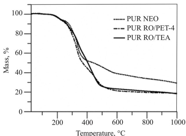
**Fig. 3. TGA results of rigid PUR foams**
