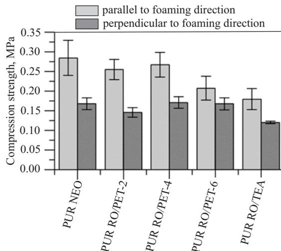
**Fig. 5. Compression strength of rigid PUR foams**
