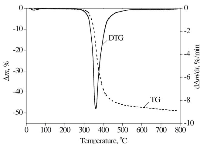
Fig. 3. Weight loss ( $\Delta m$ ) and time derivative of  $\Delta m$  ( $d\Delta m/dt$ ) curves for thermal degradation of EPY<sup>®</sup> epoxy system at heating rate 10 °C/min
