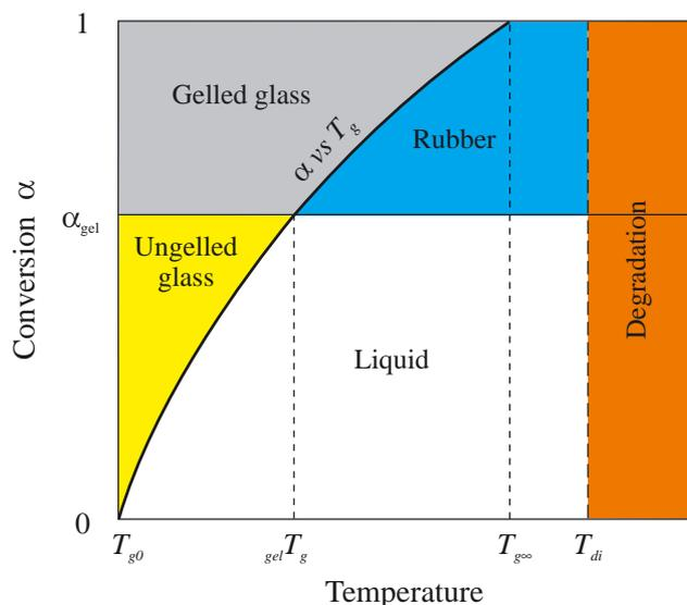
Fig. 1. Generalized conversion-temperature-transformation (CTT) cure diagram for a thermosetting system, showing four critical temperatures ( $T_{g0}$ ,  $_{gel}T_g$ ,  $T_{g\infty}$  and  $T_{di}$ ), various states of the material, and its gelation, vitrification and degradation contours
