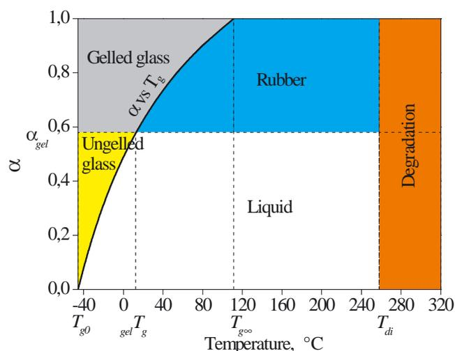
Fig. 4. Calculated CTT cure diagram for the EPY<sup>®</sup> material
