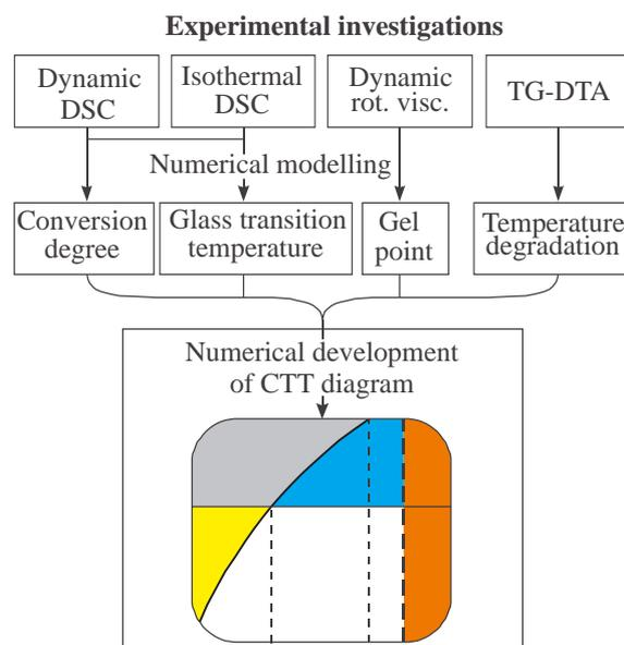
Fig. 2. Flow chart of the experimental and numerical development of CTT diagram
