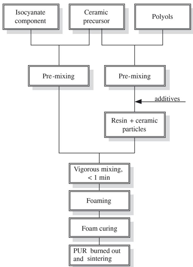
Fig. 1. Sequence of the steps of the direct foaming method to produce ceramic foams
