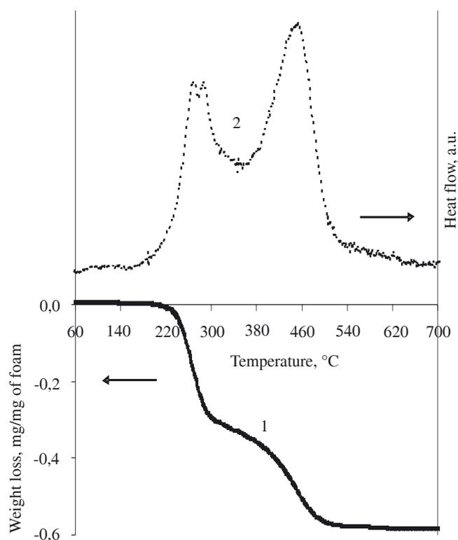
Fig. 2. Thermogravimetric (1) and differential thermal data (2) of PUR/ceramic foam E under an air flow
