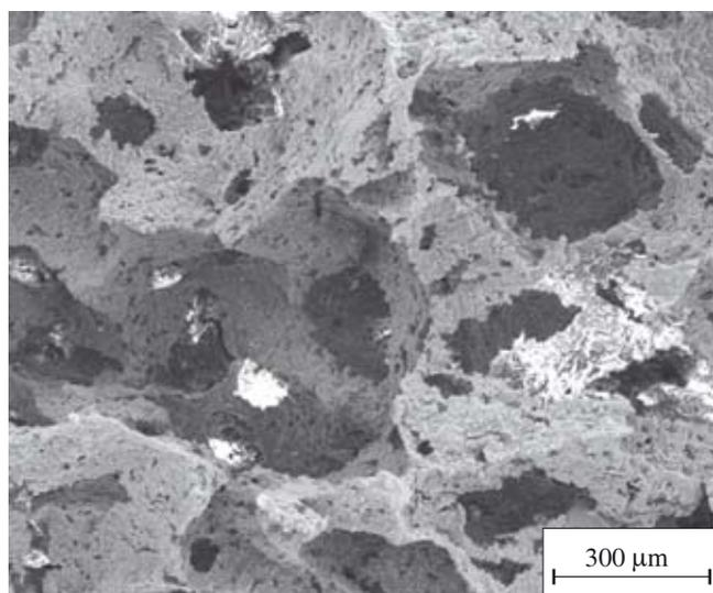
Fig. 3. SEM image of B cordierite foam
