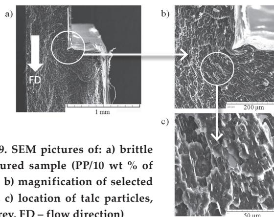
Fig. 9. SEM pictures of: a) brittle fractured sample (PP/10 wt % of talc), b) magnification of selected area, c) location of talc particles, (abbrev. FD – flow direction)
