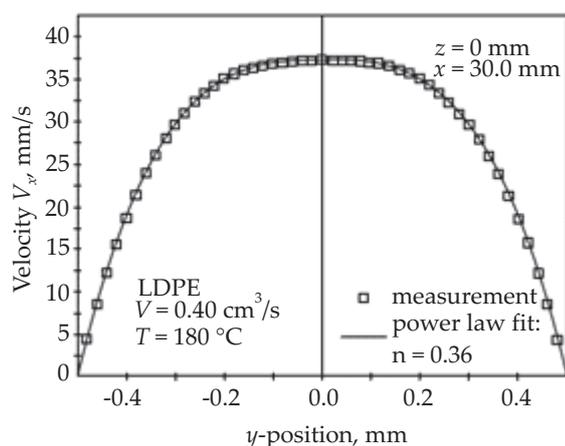
Fig. 5. The LDPE flow velocity distribution on the cross section of a die; comparison of LDV measurements with power law fit for  $n = 0.36$ ; the measurements were realized across the section of a die at the position of 30 mm after the entry from the reservoir to the die [39 similar results at 30–32]
