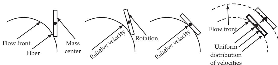
Fig. 2. Angular rate of rotation of single particle [25]
