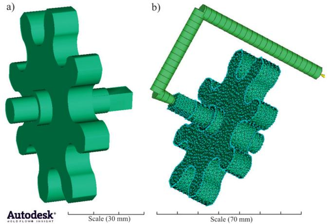
Fig. 2. Gear wheel model imported to Mflow system: a) STL model, b) FEM model with runner system
