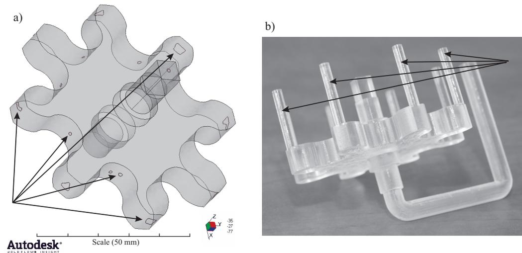
Fig. 3. Results of the mold filling simulation with air traps marked by arrows (a) and view of the master model made with stereolithographic method of adjusted shape, taking into account the results of the simulation with visible venting channels (arrows) and the runner (b)
