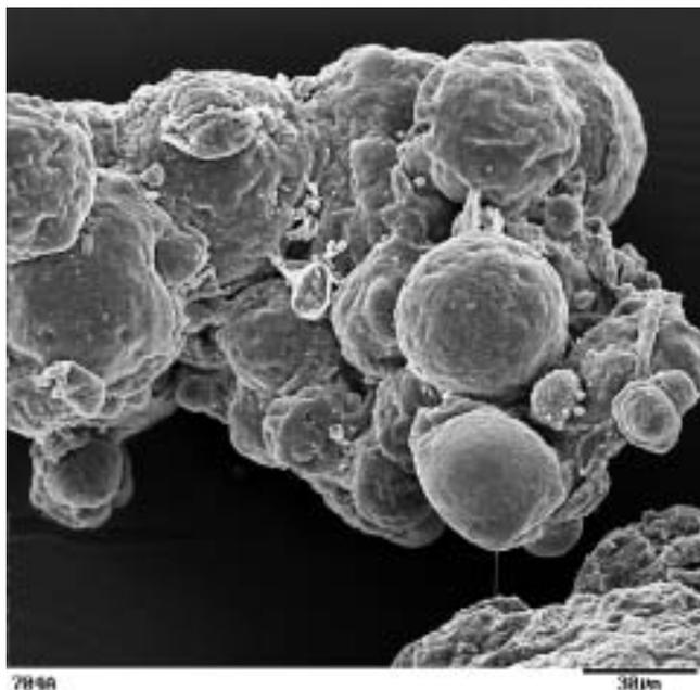
Fig. 1. SEM image of typical suspension PVC grain (control sample)
