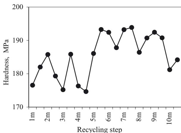
Fig. 4. Hardness changes under simulated recycling; meaning of symbols as in Fig. 1
