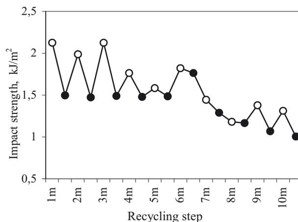
Fig. 5. Impact strength changes under simulated recycling; meaning of symbols as in Fig. 1
