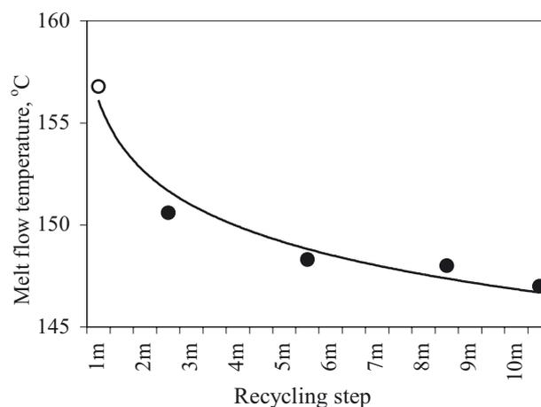
Fig. 1. Melt flow temperature changes under simulated recycling; empty circle correspond to molding steps and solid circle correspond to ageing steps
