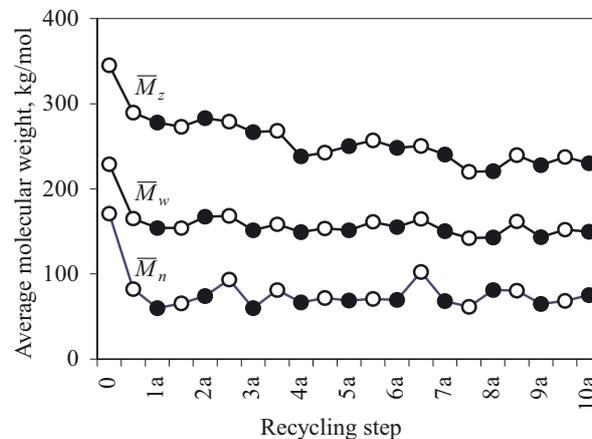
Fig. 3. Changes of average molecular weights ( $\overline{M}_n$ ,  $\overline{M}_w$  and  $\overline{M}_z$ ) under simulated recycling; meaning of symbols as in Fig. 1
