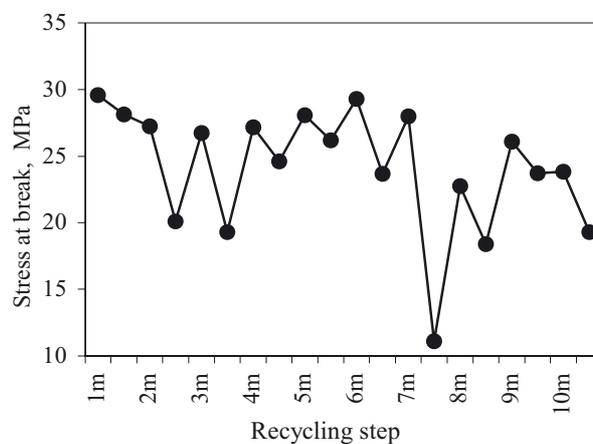
Fig. 6. Stress at break changes under simulated recycling; meaning of symbols as in Fig. 1
