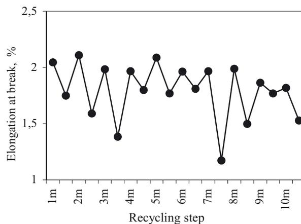
Fig. 7. Elongation at break changes under simulated recycling; meaning of symbols as in Fig. 1
